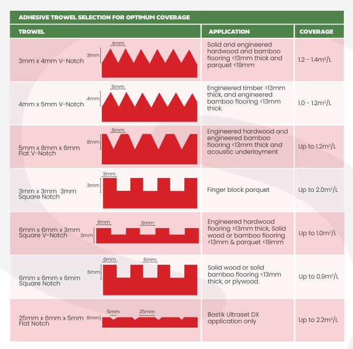
Trowel size is suggested to maximise coverage of adhesive during installation: Periodically check >80% bond area contact is achieved between flooring and subfloor. Uneven surfaces may require the use of either a self levelling / patching material, or a larger V or Flat Notch trowel for proper coverage of adhesive.
